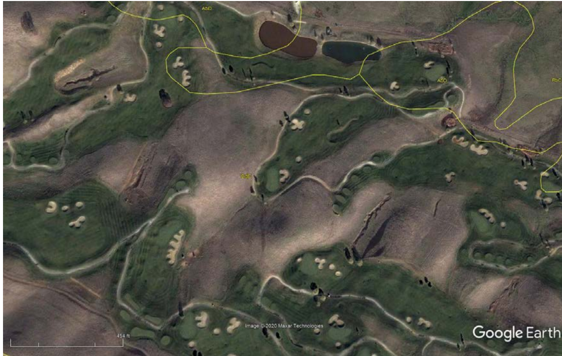
Figure 3. Overhead view of golf course soon after construction showing multiple gullies from increased runoff following grading and soil impacts. Image date: 12/13/2003.
